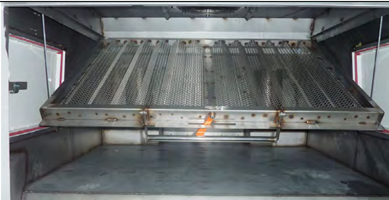
Suction fan screen lowered on its tethers
