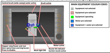
This document is designed as a quick reference quide, to allow the operator to drive the vehicle in Normal or Hydrostatic Mode and operate the basic controls. It does not constitute the full operating instructions.
