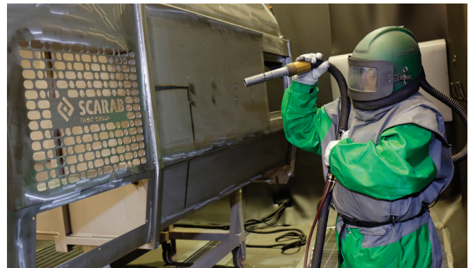
Shot blasting the stainless steel hopper
