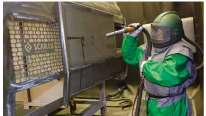
Shot blasting the stainless steel hopper
