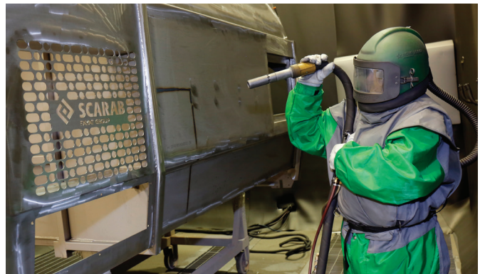
Shot blasting the stainless steel hopper
