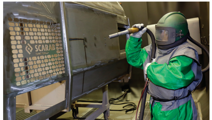
Shot blasting the stainless steel hopper
