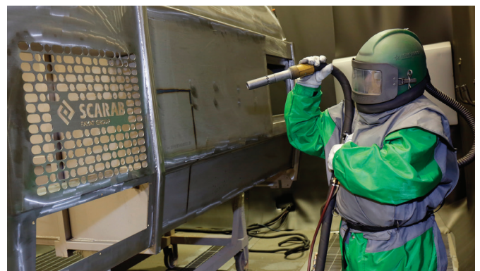
Shot blasting the stainless steel hopper
