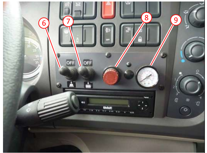
Brush pressure switches, pressure adjuster and gauge
