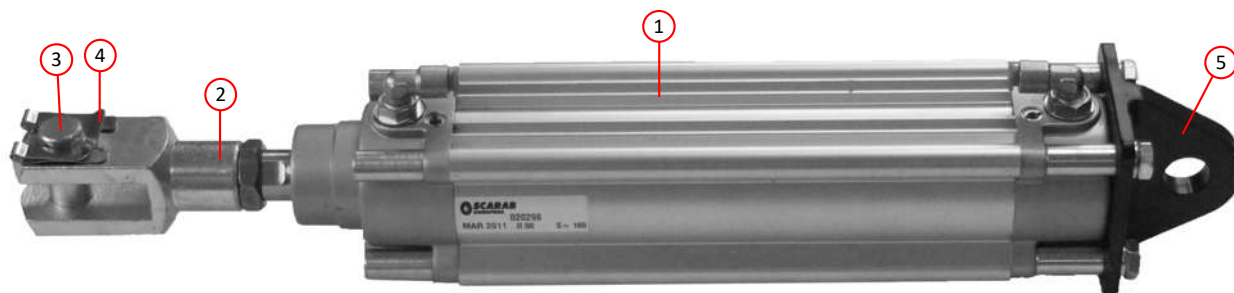
PNEUMATIC CYLINDER, SIDE BRUSH SWING IN/OUT - ASSEMBLY
