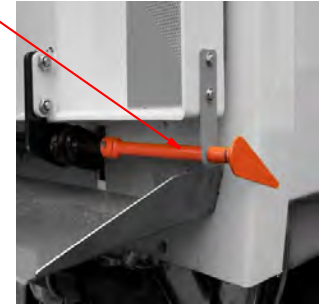
PULL TO OPEN DUMP VALVE MANUAL CONTROL
