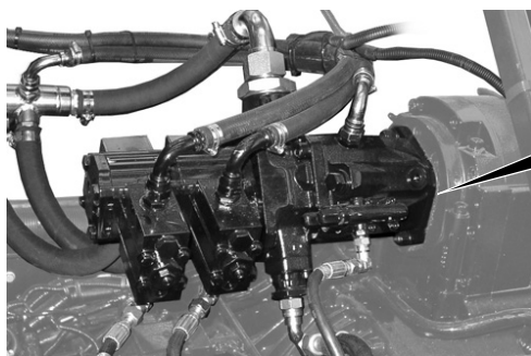
Fig. 22 The Unidrive Pumps and PTO Blanking Plate
