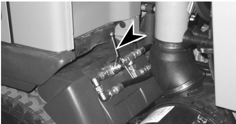
FRONT H-P SPRAY BAR CONTROL VALVE 'OFF'
