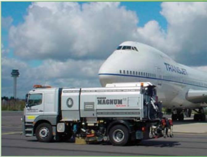
The heavy-duty Magnum Plus has all the traditional features of a Scarab Sweeper with the green and efficient single engine design which gives you greater reliability, and durability, lower emissions and lower fuel costs along with the largest payload (up to 9700 kg) and an impressive 8.8 m<sup>3</sup> hopper void.
